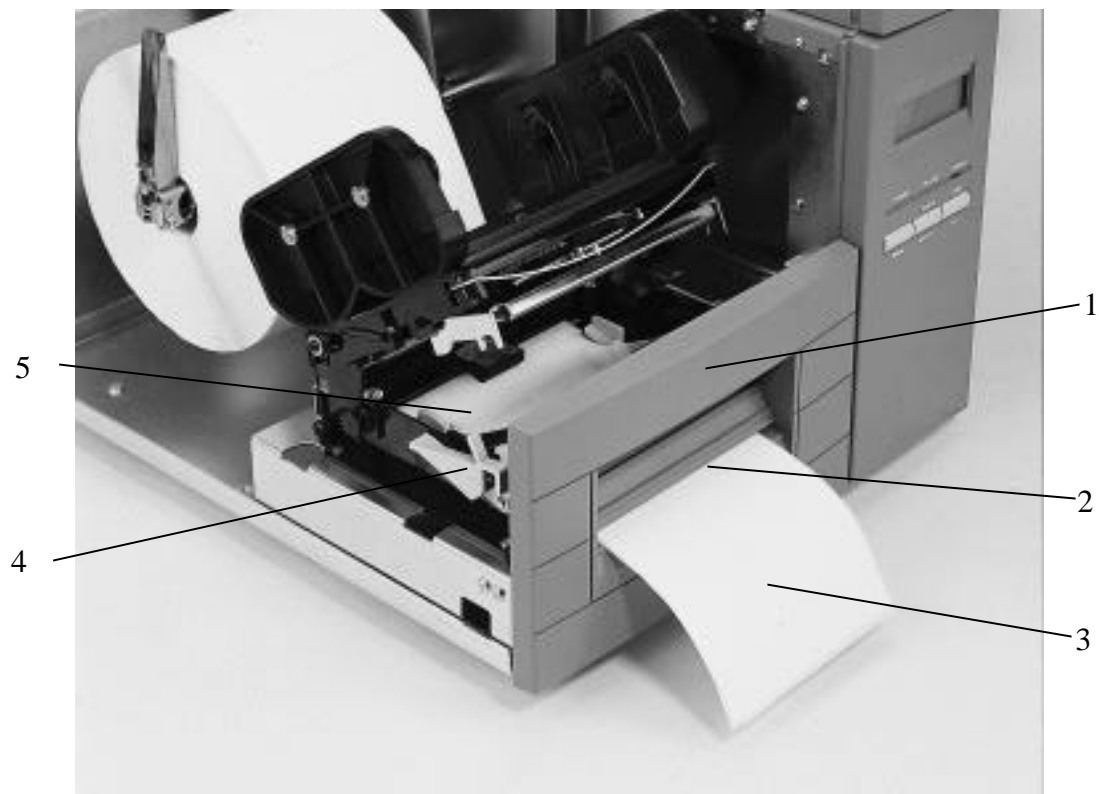
Figure 7. Printer Ready for Self-Peeling Function
