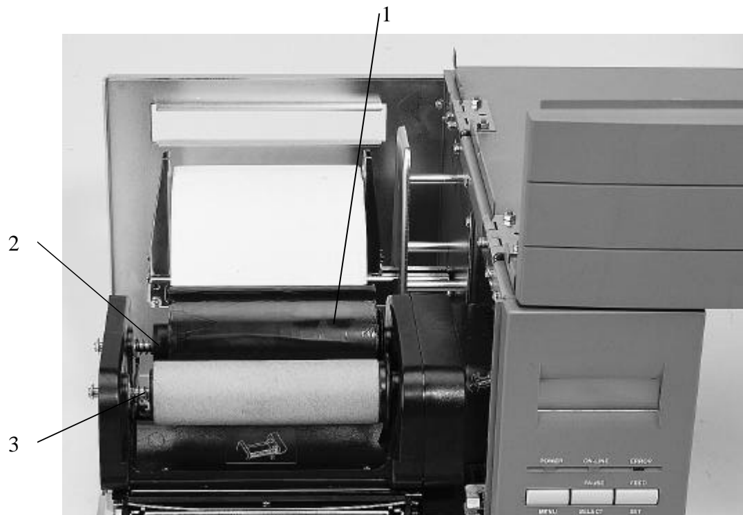
Figure 9. Placement of Ribbon Supply Roll
